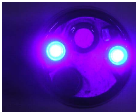
Figure 8. NBI scope after switching mode to blue light
